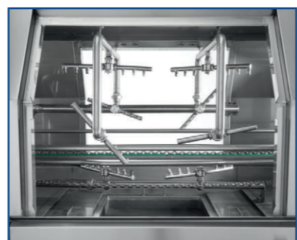
Image 23 Optimal zone length - little water/chemical carry-over
