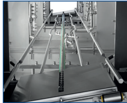
Image 17 Inclined / offset container guidance - no splash shadows
