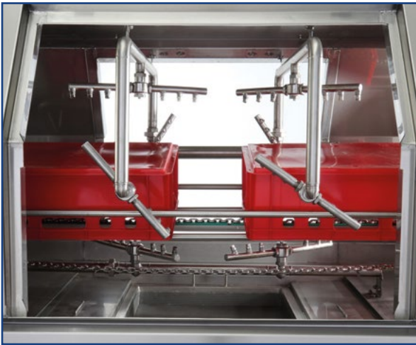
Rotary spray nozzles in the washing zone
