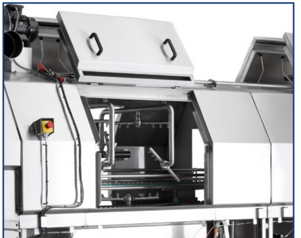
Two-phase door opening - maximum accessibility
