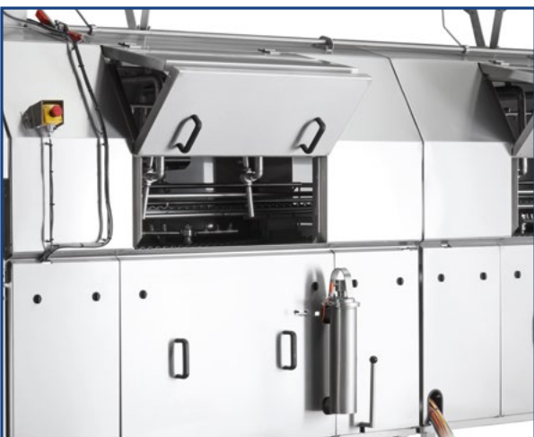
Two-phase door opening - cleaning position
